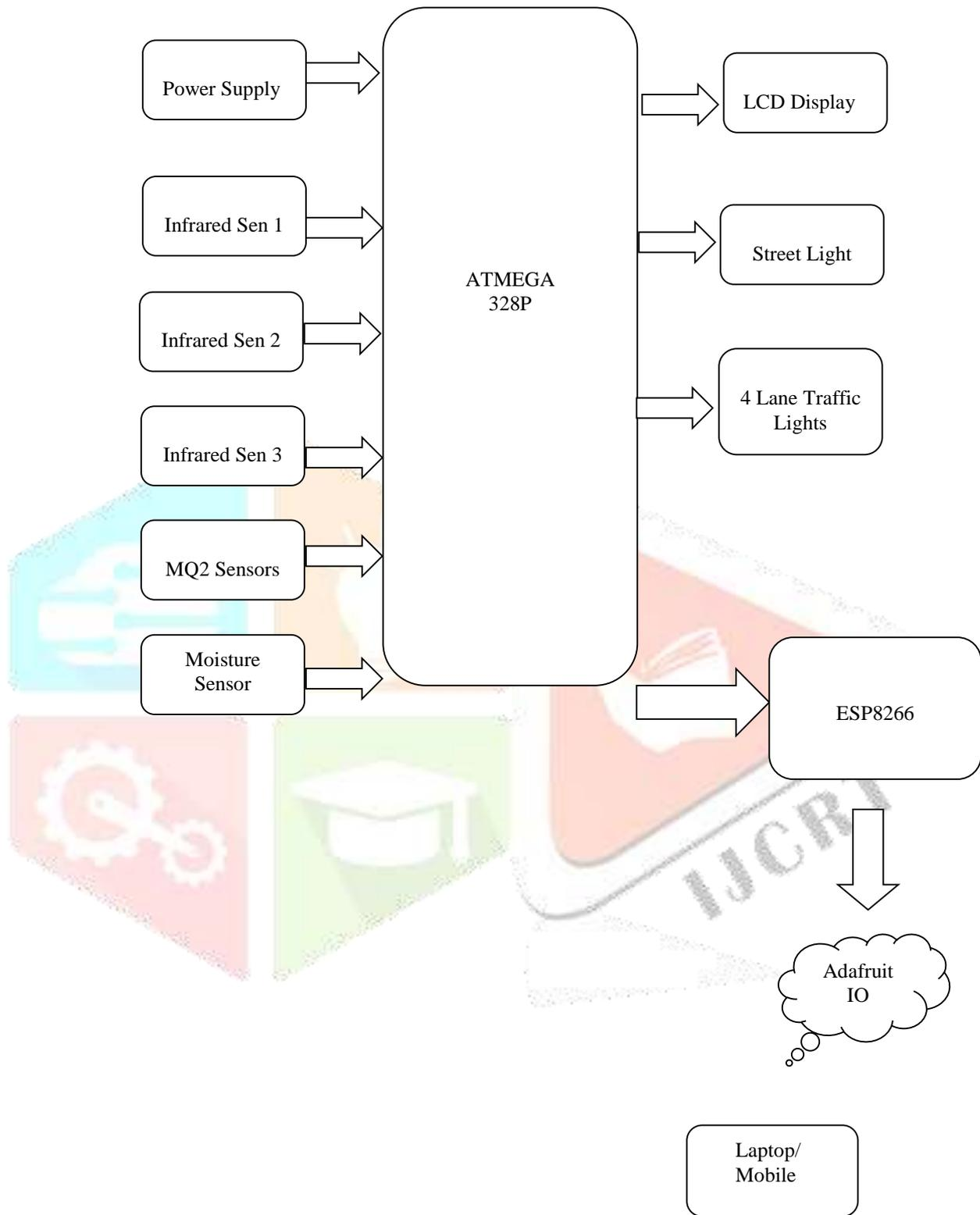
Fig 1: Block Diagram of Proposed System
