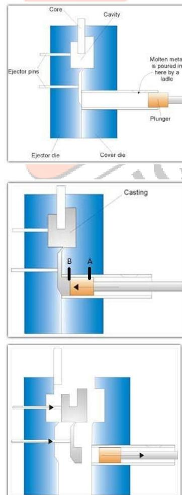
Figure 1. Steps in cold chamber die casting process, Kumar<sup>2</sup>; Han & Vishvanathan<sup>3</sup>, Domkin<sup>4</sup>
