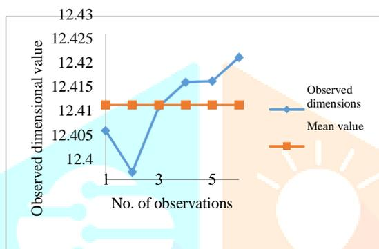
Figure 4. Run chart of the measured values of outer diameter.
