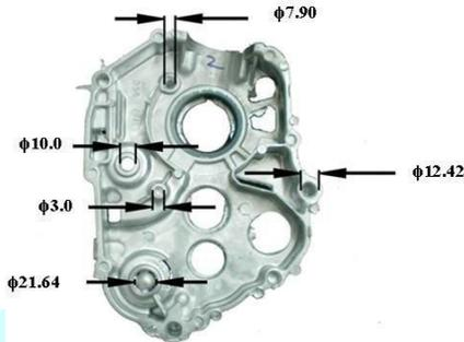
Figure 3. Bench mark for cold chamber die casting (all dimensions in mm).
