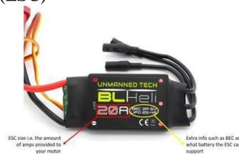
The drone requires four 30 Amp Esc controllers to control the speed of the BLDC motors. An electronic speed control (ESC) is a circuit that regulates and controls the rotational speed of an electric motor. It may also be capable of motor reversing and dynamic braking. In electrically powered radio-controlled models, miniature electronic speed controllers are used.
