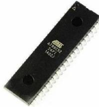
The AT89C52 is a low-power, high-performance CMOS 8-bit microcomputer with 8K bytes of Flash programmable and erasable read only memory (PEROM). The device is manufactured using Atmel's high-density non-volatile memory technology and is compatible with the industry-standard 80C51 and 80C52 instruction set and pinout.
