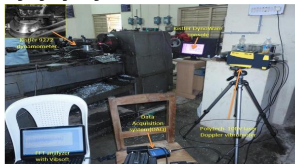
Fig. 3 Experimental setup used for Face Turning
