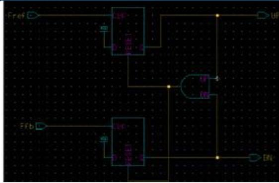
Figure 4.4 Block diagram and schematic diagram of PFD.
