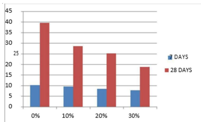
**Compressive strength of M<sub>25</sub> grade concrete cubes after 7 days**
