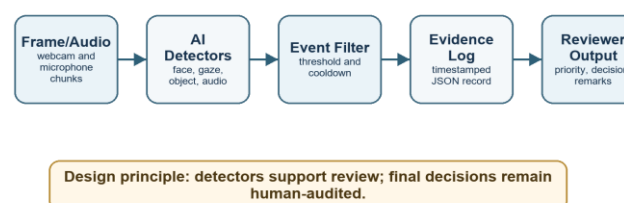
Fig. 2. Evidence generation workflow from detector signal to reviewer output.
