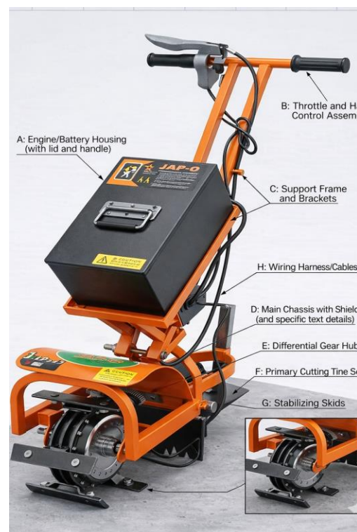
Fig. 2. Electric Cultivator Made by Hand — 3D View This view shows all the main parts (A through H).
