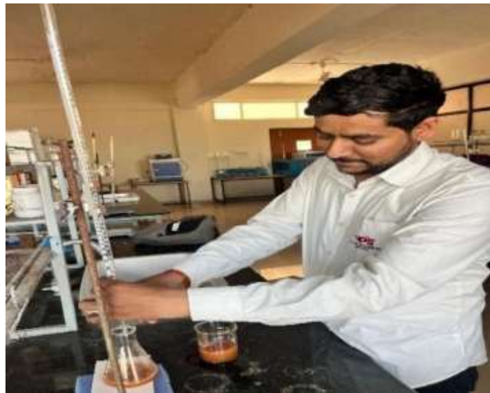
Hardness test on a raw waste water sample
