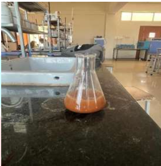
Chloride test on raw waste water sample
