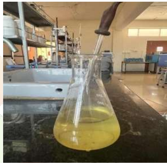
Chloride test on raw waste water sample
