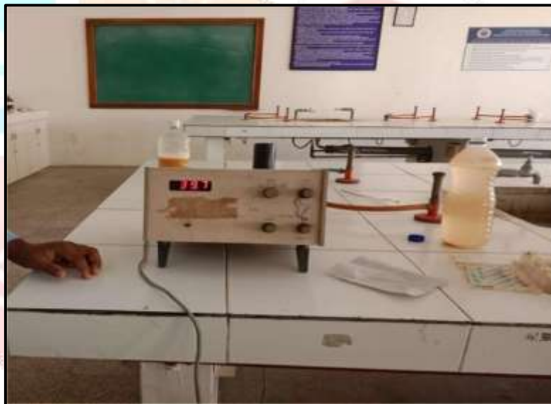
Turbidity test on a combination neem leaf powder, aloe vera gel
