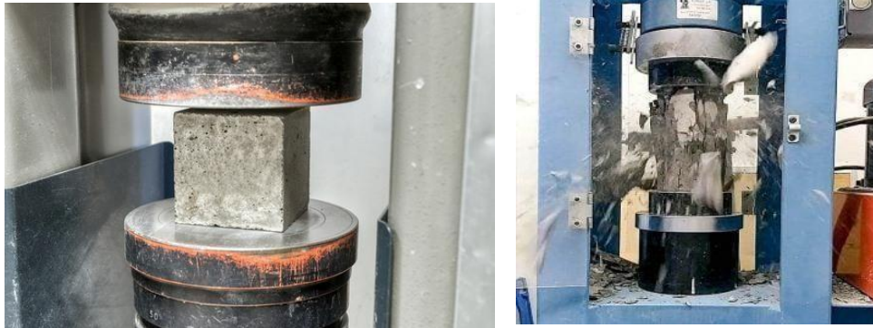
Compressive Strength Test
