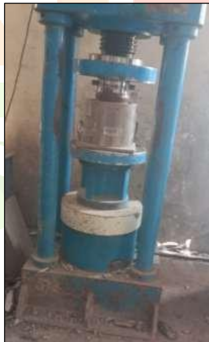
Fig.06. Aggregate crushing test
