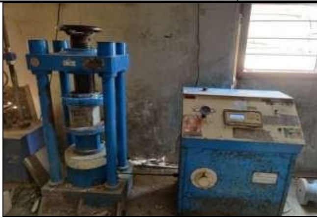
Fig.13. Cube testing machine
