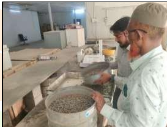
Fig.02 - Moisture content in Aggregate
