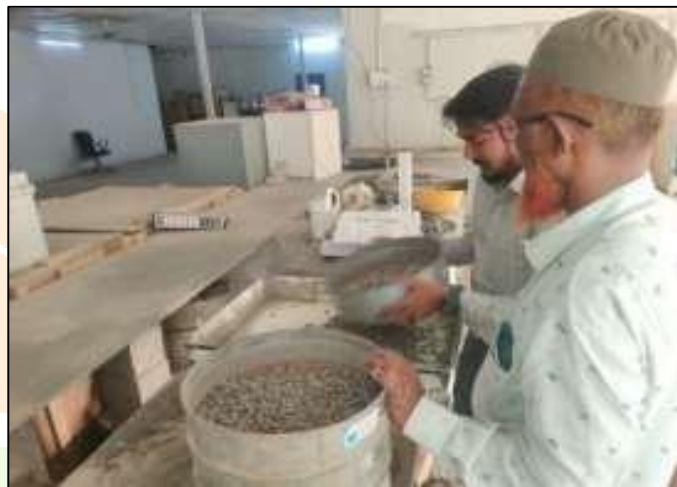
Fig.02 - Moisture content in Aggregate
