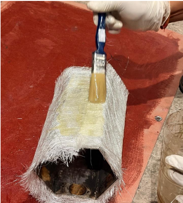
Fig.33 Application of Glass Fiber Layer using resin solution.
