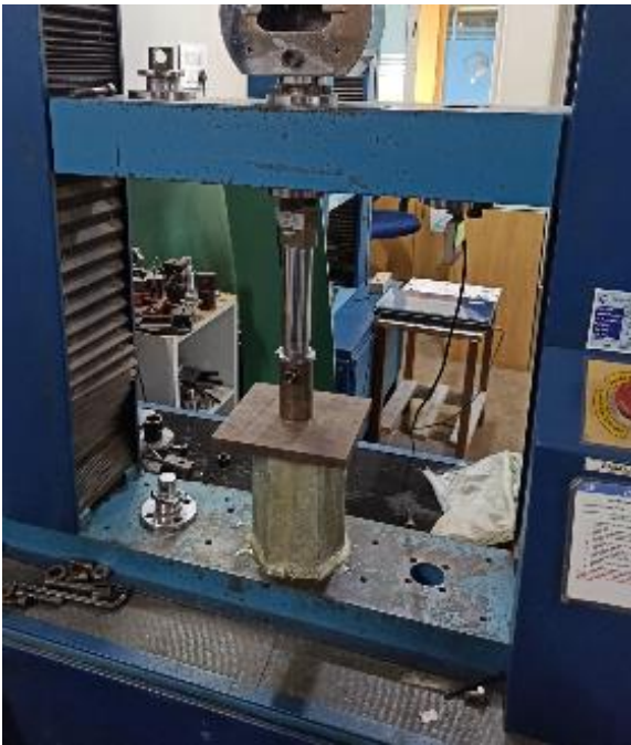
Fig.36 Specimen under compression testing using UTM.
