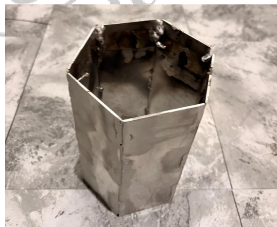
Fig. Aluminium Hexagonal Crash box before Glass Fiber Reinforcement.
