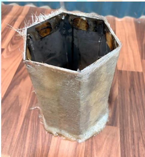
Fig.34 Final Glass Fiber Reinforced Specimen.
