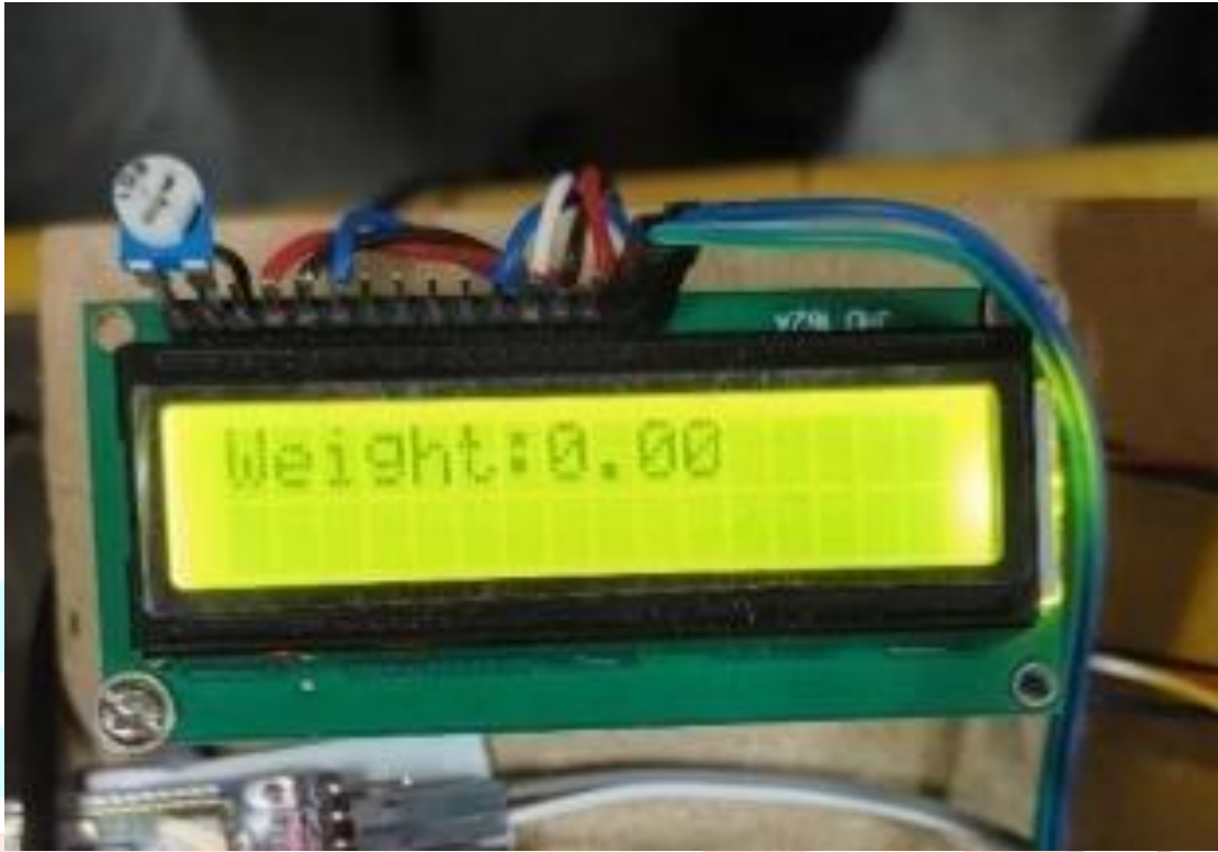
Fig.9. Measuring the initial weight for theft detection
