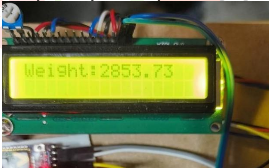
Fig.9. Measuring the initial weight for theft detection
