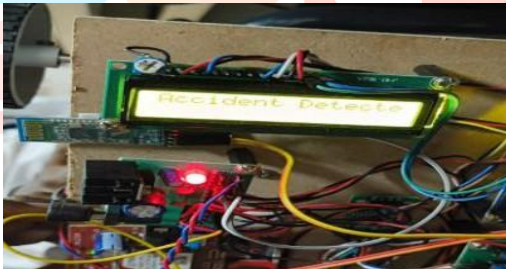
Fig.12. Display indicating that an accident has been detected based on the tilt angle
