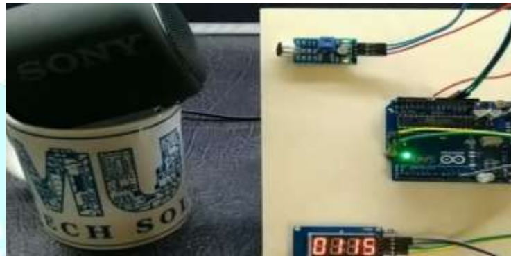
Fig 5.1: Result1 (sound measured is above 85Db)
