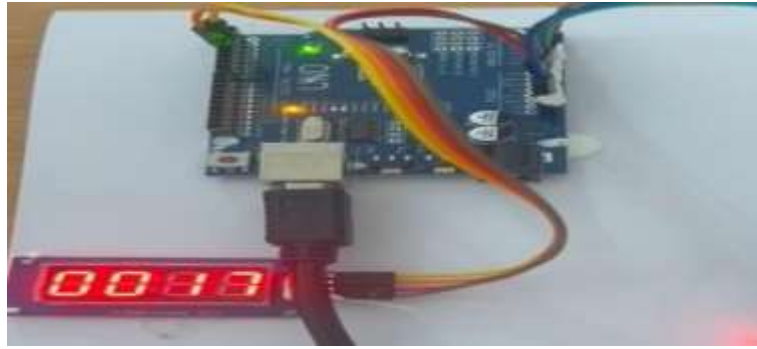
Fig 5.1: Result1 (sound measured is below 85Db)
