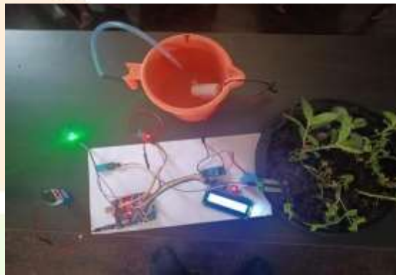
Fig 5: Model of automatic plant watering system
