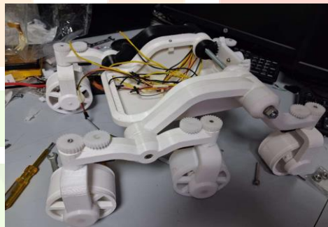
Fig. 1: Hardware assembly of the autonomous surveillance robot showing the six-wheel drive chassis, DC geared motor mounting, and initial electronic component placement during the fabrication phase.
