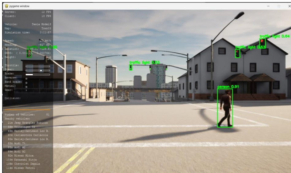
fig. 6. output sample of the YOLO v5 Object detection model highlighting “person” (a pedestrian) and multiple “traffic light” at a cross section
