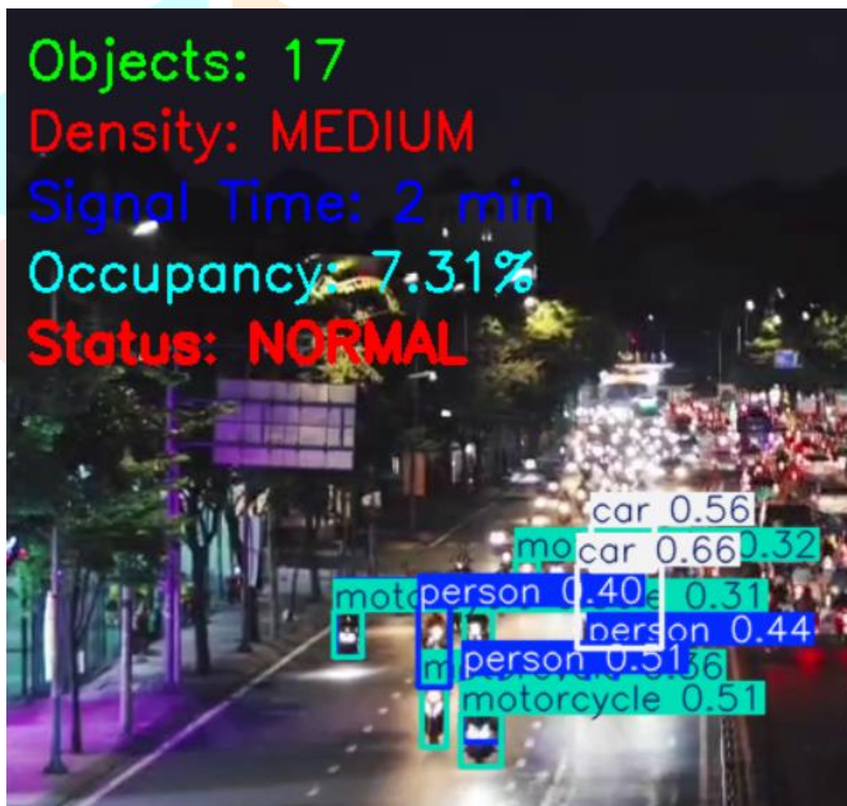
Fig. 2: Integrated Output of Traffic Density, Occupancy, Congestion Classification, and Adaptive Signal Timing
