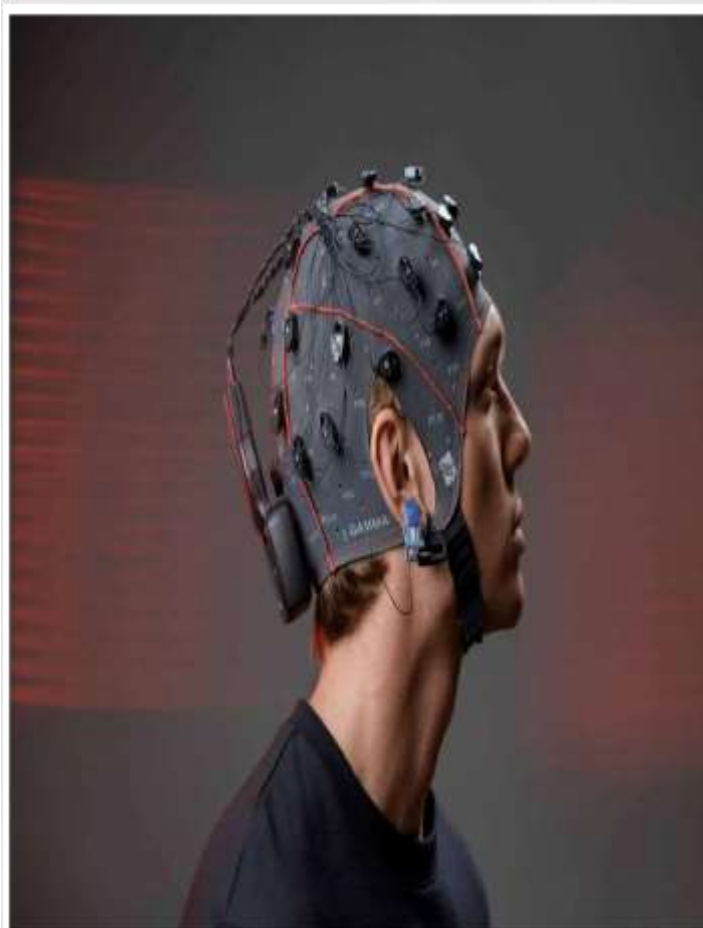
Fig. 4. High-density EEG system for cognitive state monitoring. Advanced dry-electrode arrays enable non-invasive brain-state classification, supporting applications in cognitive load monitoring, attentive augmentation, and mental wellness BCI.
