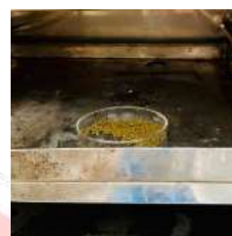
fig. 6 Drying of granules
