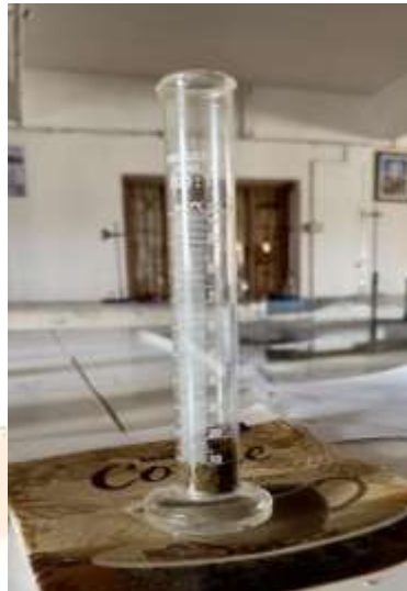
fig. 10 measuring cylinder for tapped density
