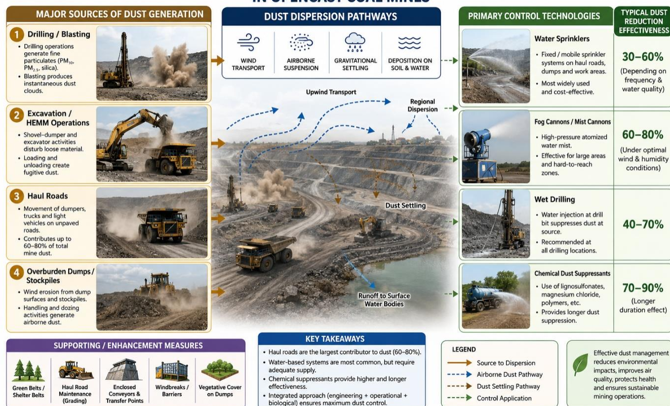
Figure 1: Major Sources of Dust Generation and Primary Control Technologies in Opencast Coal Mines
