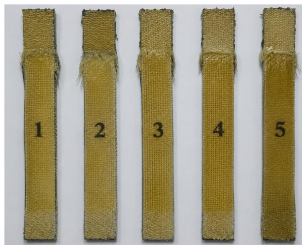
Fig 1: Tensile test specimens (Specimens 1–5) and their dimensions as per ASTM standards
