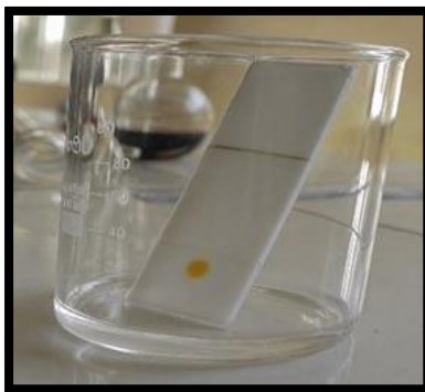
Fig 4. Thin-Layer Chromatography (TLC) of the Benzoxazole-Thiazole Hybrid
