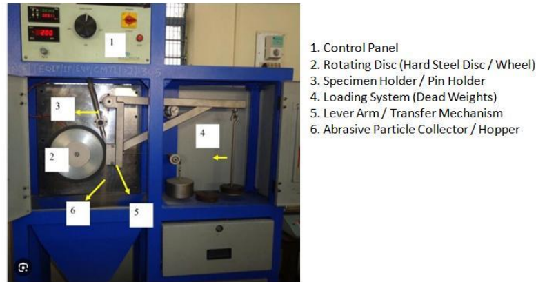
Figure 3.2: 3-Body Abrasive Wear Testing Equipment
