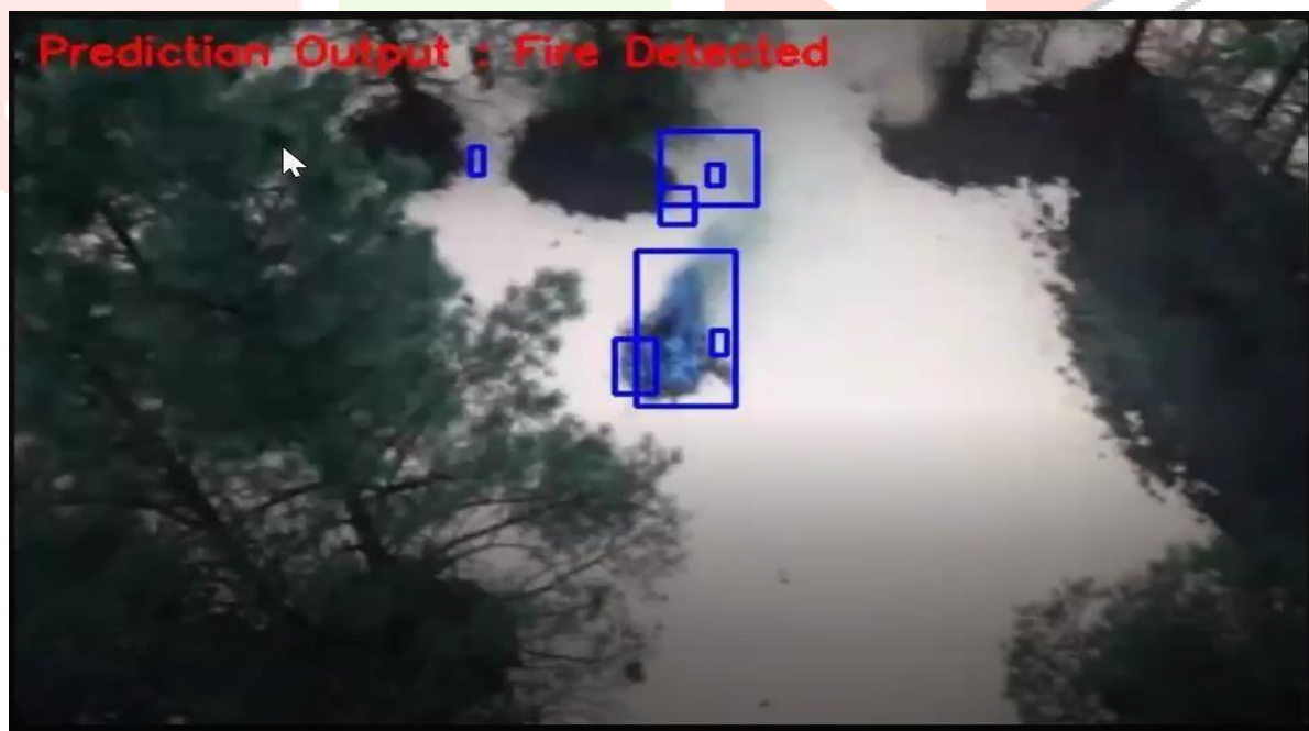
Figure 10: Detected Fire Regions in Forest Image Using CNN Model
