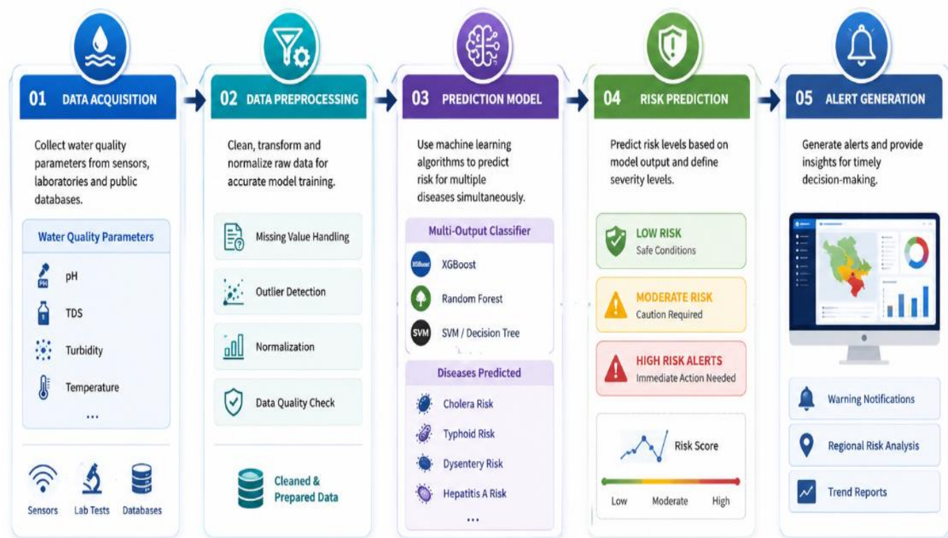
Fig 1: System Architecture of the Smart Community Health Monitoring and Early Warning System for Water-Borne Diseases
