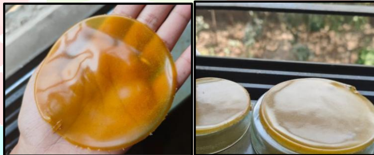
Fig no. 03. orange pectin based bioplastic film
