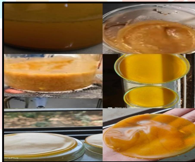
Figure no 02. process of bioplastic film
