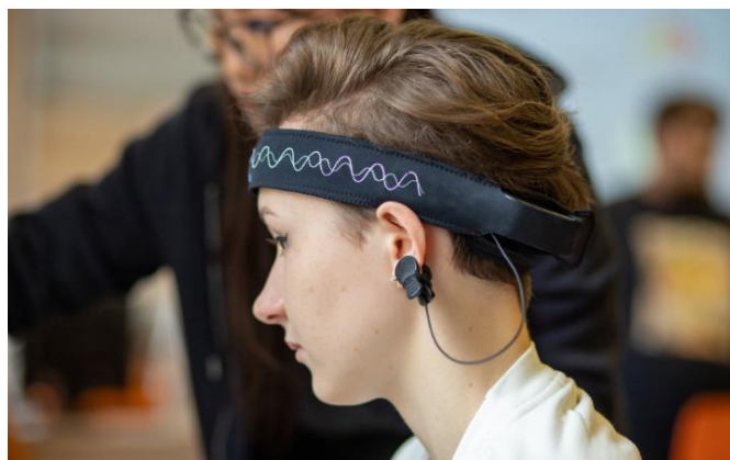
Figure 3. EEG-Based Smart Headband for Neuromorphic Brainwave Monitoring in Meditation and Cognitive Wellness Applications
