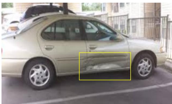
FIG 9.1a: Moderate Damage — Detected Region (Bounding Box)
