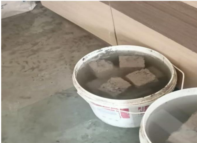
Fig no.5: Immersion of cubes in acid
