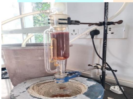
fig 01:(drug extraction process with the help of soxhlet apparatus)
