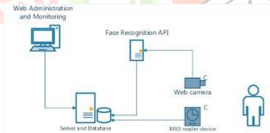
Fig: RFID and face recognition system Architecture
