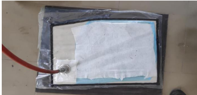
Figure 3 Vacuum bagging of fabricated plates
