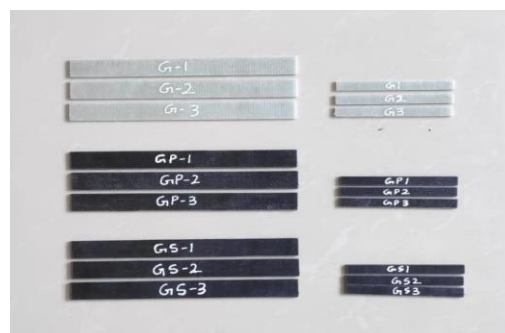
Figure :5 Cut specimens for tensile and flexural testing
