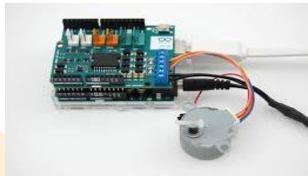
Fig:8 final hardware circuit of stepper motor
