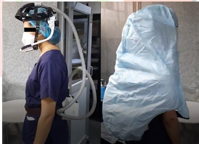
Figure 6. (A) Assembled PAPR system, (B) Helmet gear and waist gear donned by the healthcare worker, (C) device covered under the PPE kit hood.
