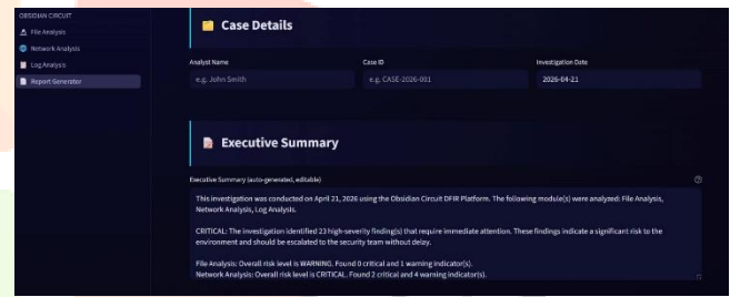
Figure 18. The interface of a Report Generator, which involves the input of the case details into the interface by the analyst (name and ID). This view gives an auto-generated, editable Executive Summary that summarizes the total number of critical and warning indicators across the investigation of their analysis modules associated with File, Network and Log analysis modules.
