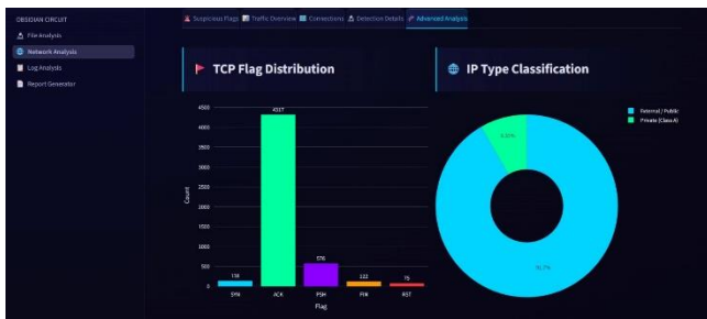
Figure 12. Advanced Analysis dashboard with the visual telemetry of the network traffic. The interface presents a TCP Flag Distribution histogram, and IP Type Classification donut chart (with 91.7% External/Public traffic), which enables you to quickly identify an unusual scanning behavior or external connection without authorization.
