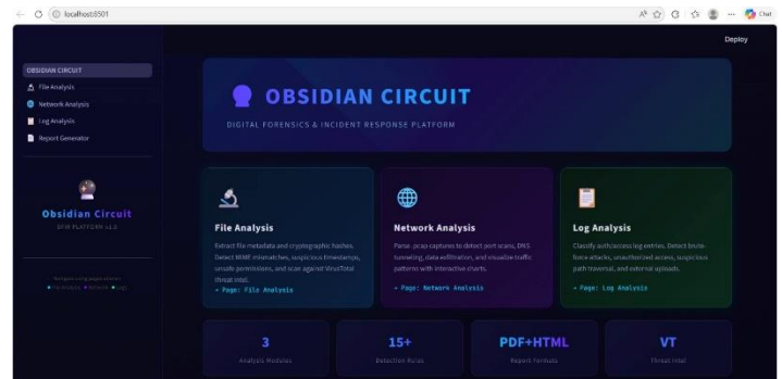
Figure 1. The main dashboard interface of Obsidian Circuit, displaying the three integrated forensic modules: File Analysis, Network Analysis, and Log Analysis. The dashboard provides investigators with a centralized interface to navigate between modules, review available analysis capabilities, and initiate forensic investigations carefully.
