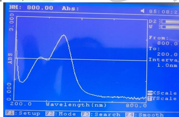
Figure 2: UV-Vis absorption spectrum after pH adjustment, demonstrating reduced intensity and broadened profile in Batch 1 (pH 5.0) indicative of particle aggregation, contrasted with well-defined absorption in Batch 2 (pH 8.2).
