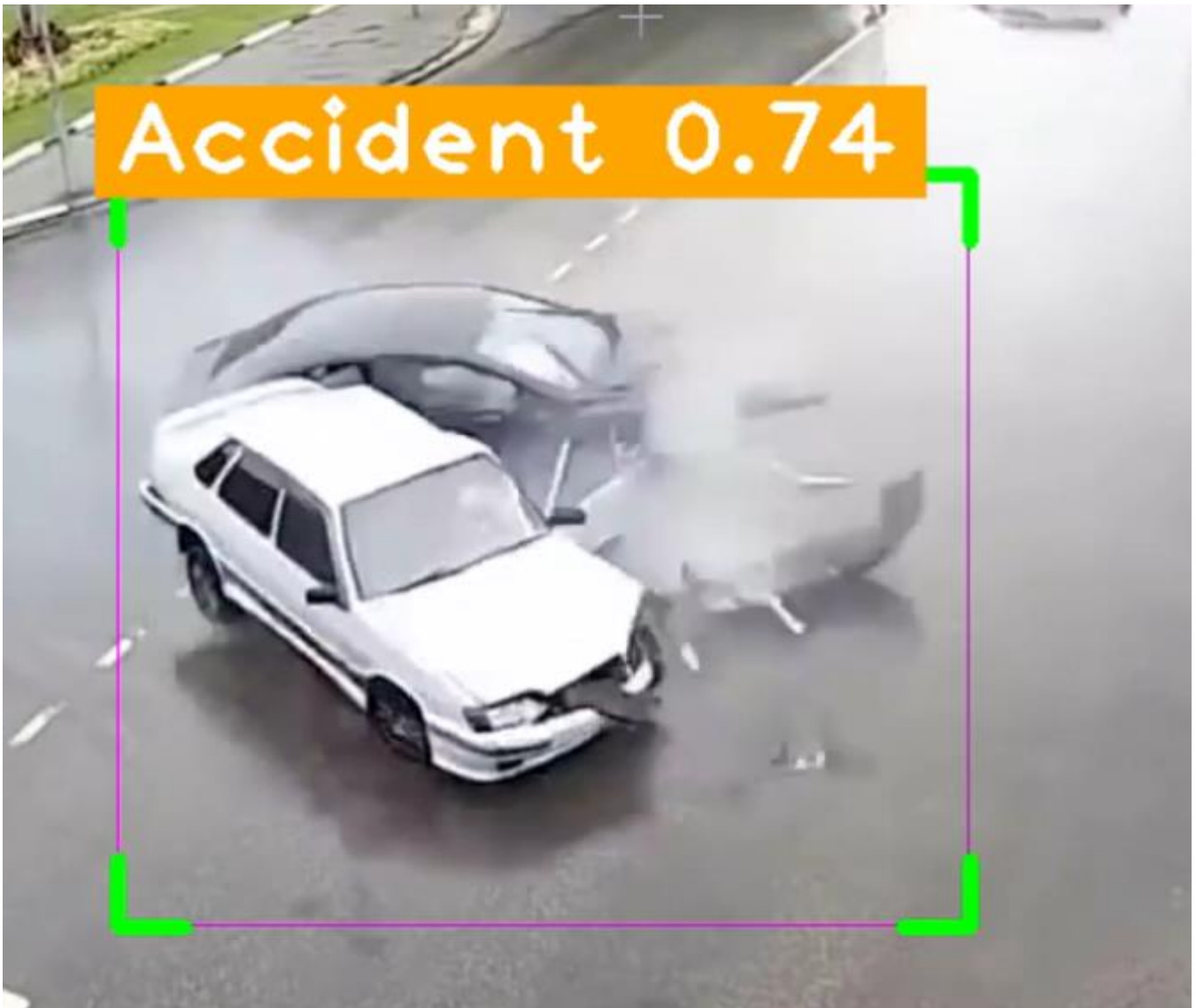
Fig. 4 detection output showing YOLOv8 bounding boxes annotated with confidence scores and SORT tracking ids on a highway collision frame.
