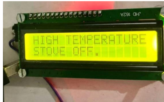
Fig 3. LCD display showing high temperature
