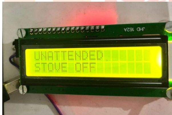
Fig 4. LCD display showing unattended stove alert
