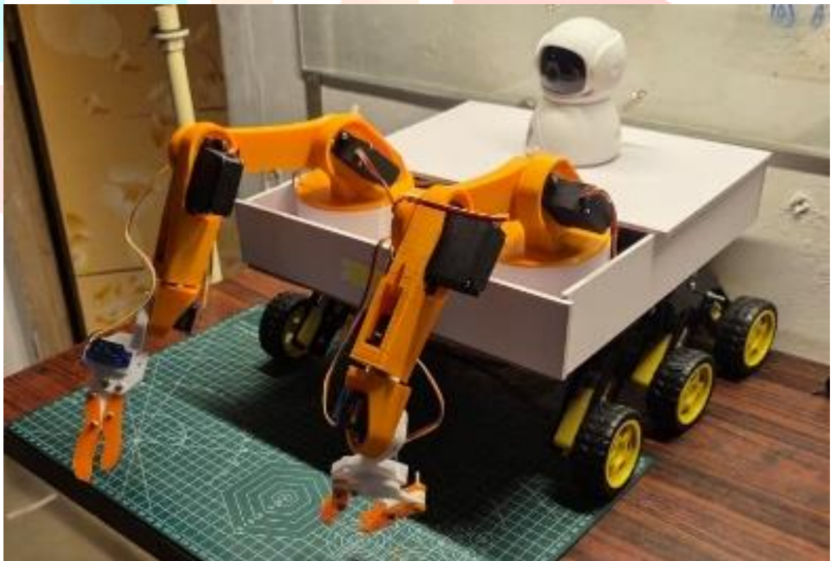
Figure 6. Front-angular view showing the rocker-bogie stance and 3D-printed grippers.
