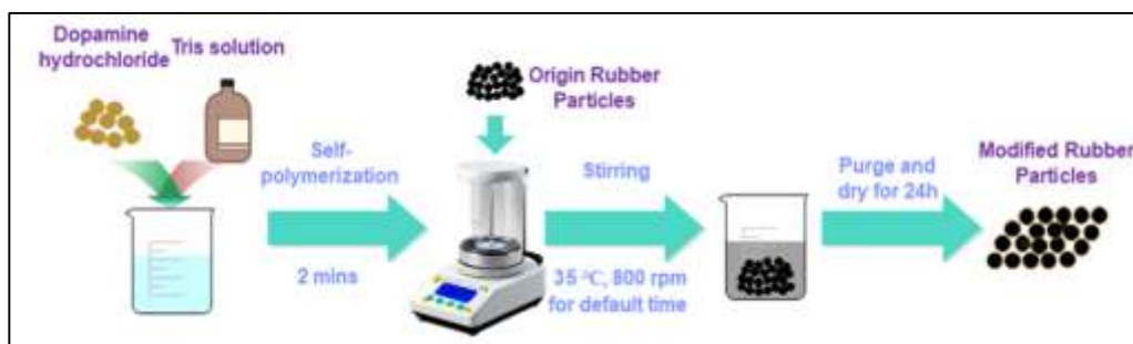
Figure 3: Process of Crumb Rubber Surface Modification [26]
