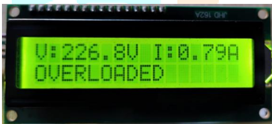
Fig 8. Overloading Result in both Hardware and Software
