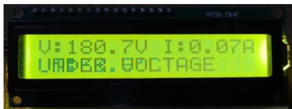
Fig 6. Voltage error Result in both Hardware and Software
