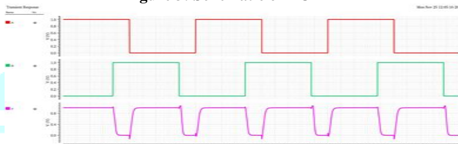
Figure 4: Same frequency, 135 degree phase shift of B
