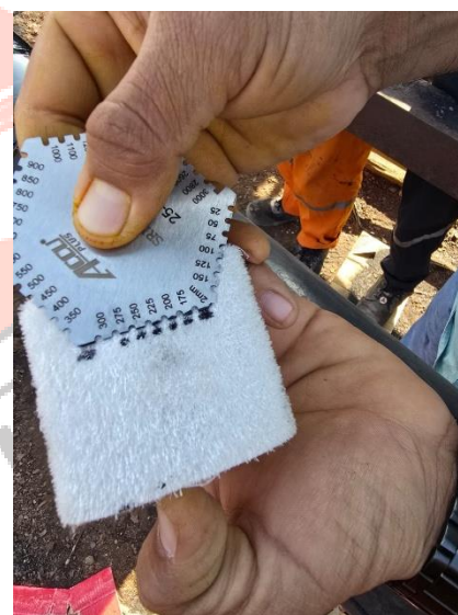
Fig 3.7 – Thickness Measure by Wet Film Thickness Gauge
