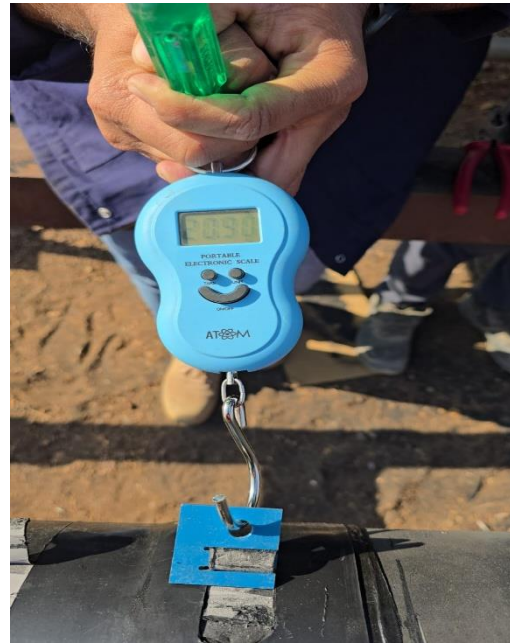
Fig 3.11 – Peel Test for proper Adhesion
