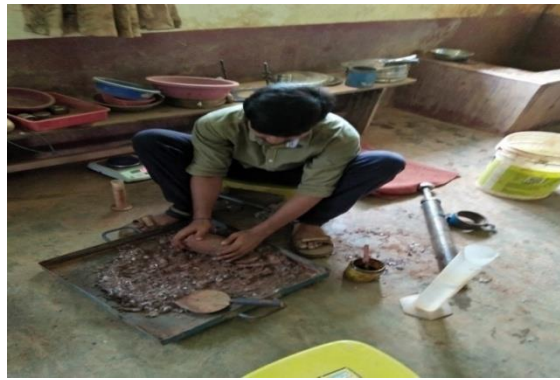
Figure: 4.5 Compaction of the PF
