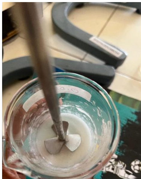
Figure 22: Mixing of face serum by using propeller
