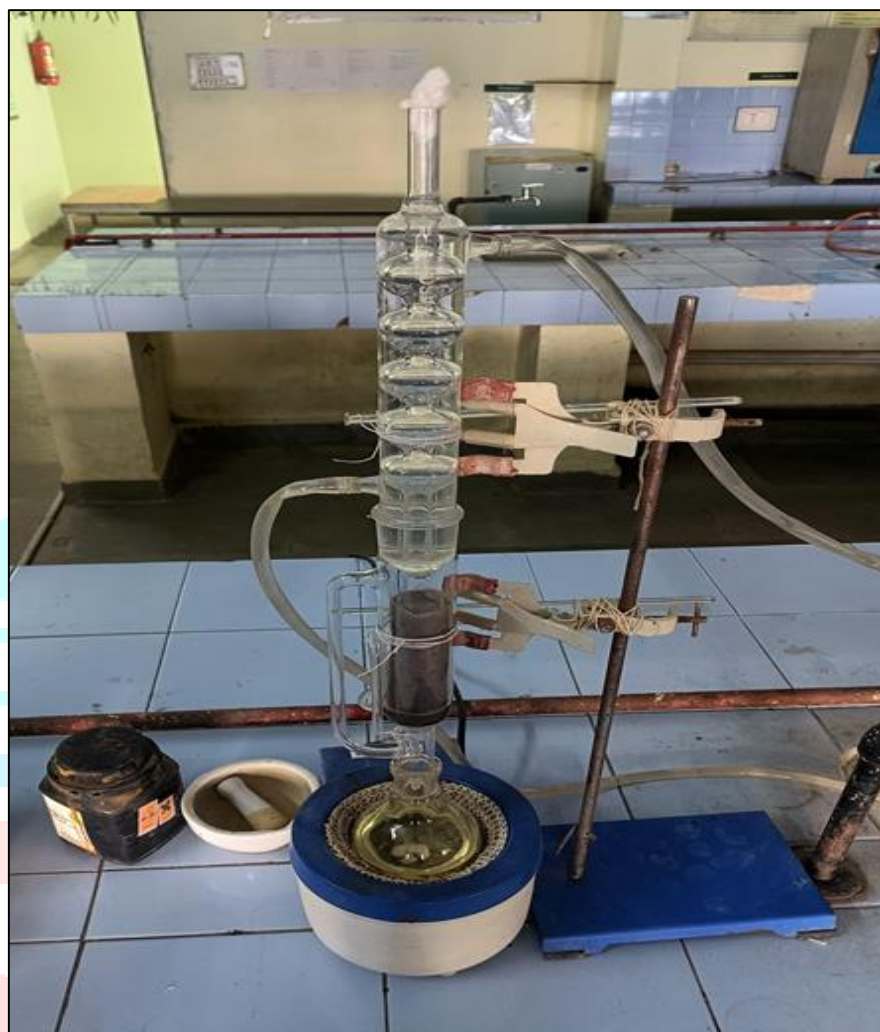
Figure 5: Soxhlet Apparatus for Successive Solvent Extraction
