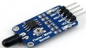
Fig shows the IR Flame Sensor. The IR flame sensor senses the environment and detects the presence of fire or flame. The module is based on the IR receiver and basically detects the presence of flammable and harmful gases like nitrogen, hydrogen, carbon monoxide. The signal detection capacity is adjustable. The robot contains three flame sensors
