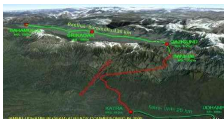
Fig 1: Alignment of the railway line
